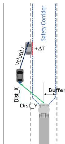
Figure 9. Overview of distances and variables for kinematic calculations. The vehicle on the left lane requires  $\Delta T$  time, corresponding to  $TT_{cross\_border}$ , to cross into the safety corridor on the ego-lane in front of the ego-vehicle.
