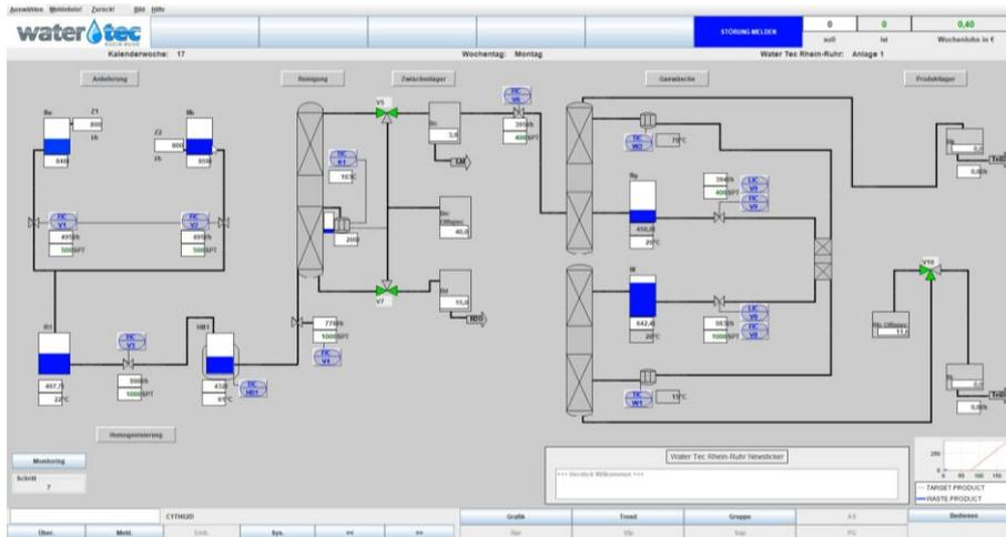
Figure 1. Screenshot of WaTr Sim with valves (e.g. V1, V6), heaters (e.g. H1, W1) and tanks (e.g. Ba, Bc).
