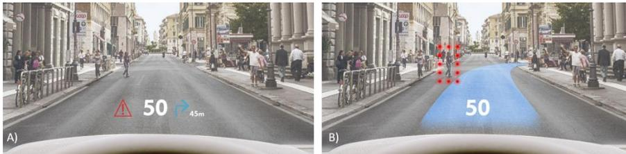
Figure 1. Comparison of a conventional HUD and an AR-HUD showing speed information, a navigation cue and an obstacle warning.
