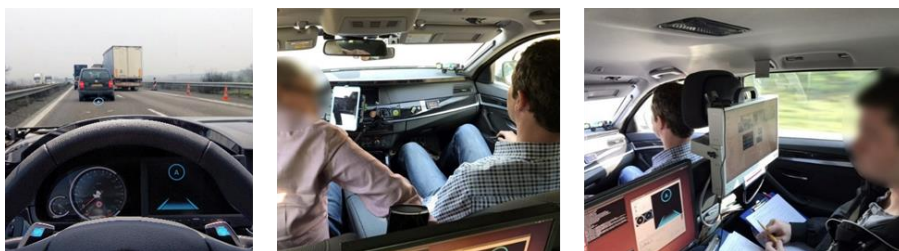
Figure 2. Automation related HMI (left); co-driver as driver wizard (middle); experimenter as HMI wizard on the back seat (right). Figure adopted from Naujoks et al. (2018).
