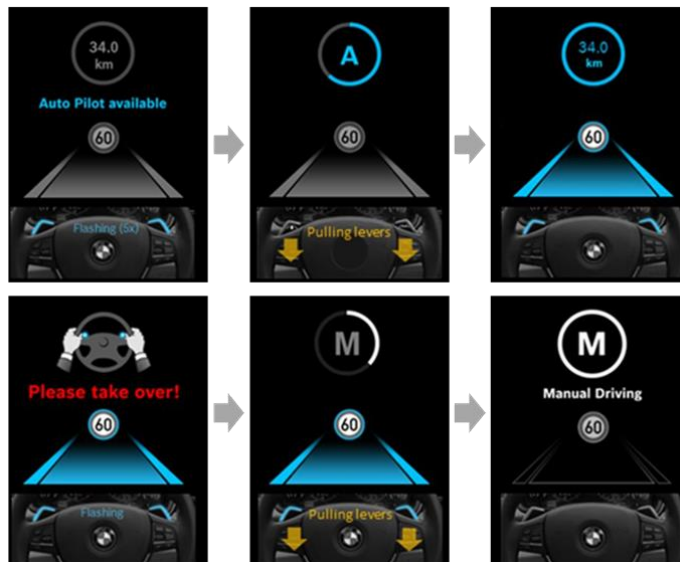
Figure 3. Visual HMI display for activation (top) and deactivation after RtI (bottom). Control transitions were generally signaled by acoustic signals with dedicated speech messages. Figure adopted from Naujoks et al. (2018).
