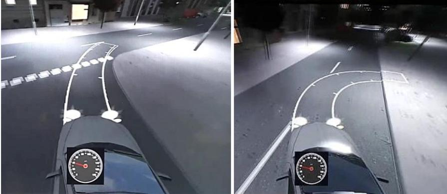
Figure 5. Light band of the “trajectory display” overlapping with lane markings (left) and the side walk (right).
