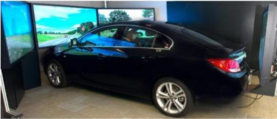
Figure 4. Fixed-base driving simulator at Opel Automobile GmbH.
