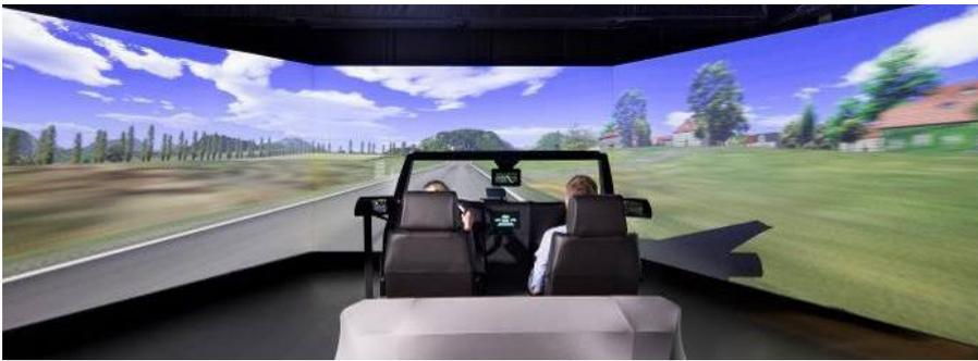
*Figure 1. The driving simulation lab with the fixed-base mock-up and 190° view of rural driving environment.*
