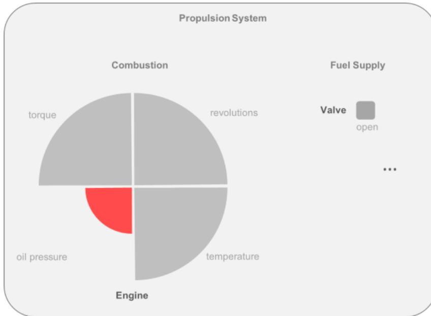
Figure 5. Example Glyph for engine.
