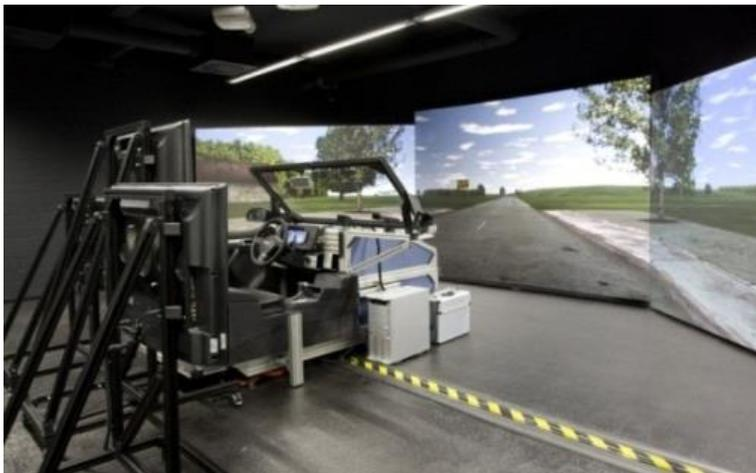
*Figure 3. Static driving simulator of the Group Research of Volkswagen AG*
