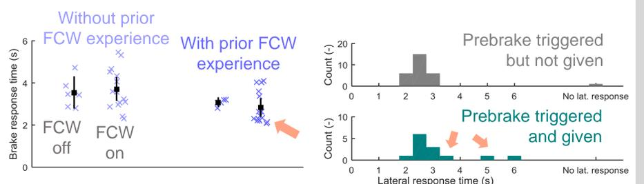
Non-significant interaction, brake response in unexpected scenario: FCW useful only for FCW-experienced drivers, even detrimental for the rest?
