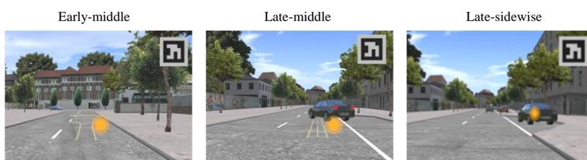
*Fig. 3: The three warning signals examined in study II: (left) early warning signal presented in the middle of a HUD; (middle) late warning signal presented in the middle of a HUD; (right) late warning signal presented sidewise in augmented reality.*
