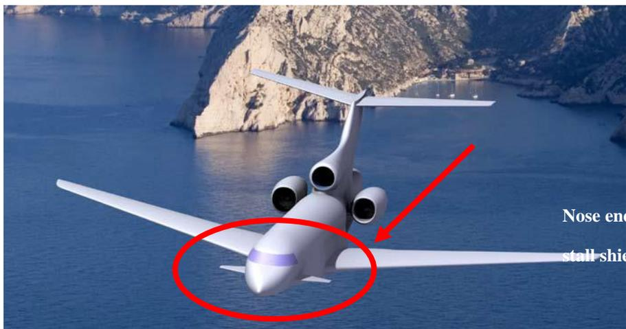
**Figure 3. Stall shields at the nose end of a T-tailed aircraft (This figure is taken from Flight Path 2050, Europe’s Vision for Aviation. Report of the High Level Group on Aviation Research. European Union 2011.)**
