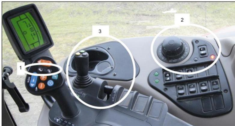
**Figure 3.** The 3-point linkage fast switch (1), the 3-point linkage control (2), and the hydraulic system (3)
