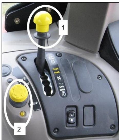
**Figure 2. Lever (1) and knob (2) controlling the PTO**
