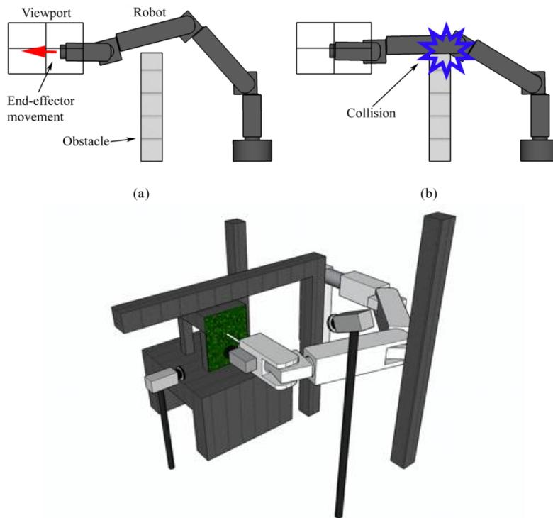
*Figure 1 Robotic arm tele-operation is affected by limited field of views and cluttered environments. Human performance challenges increase in cluttered environments.*
