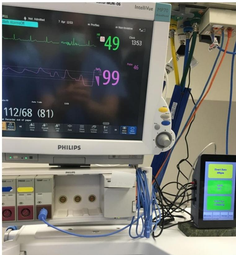
Figure 1. Music Volume Controller Interfaced with Anaesthesia Monitor. The photo shows the position of the music volume controller next to the anaesthesia monitor. The heart rate of 49 beats-per-minute triggers a music volume reduction and this is indicated by a colour change on the controller screen from green to yellow.
