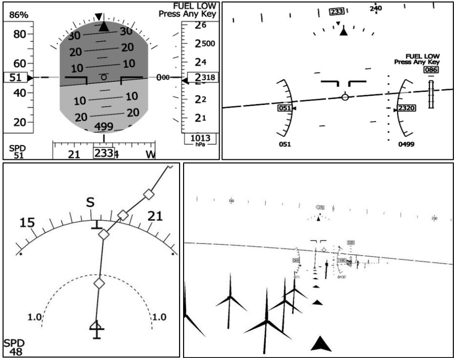
Figure 2. Head-down displays (left) and helmet-mounted display (right). Primary flight displays (top) and navigation displays (bottom).
