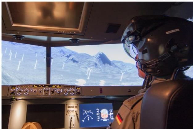
Figure 1. Generic Cockpit Simulator (GECO) and JEDEYE™ helmet system.
