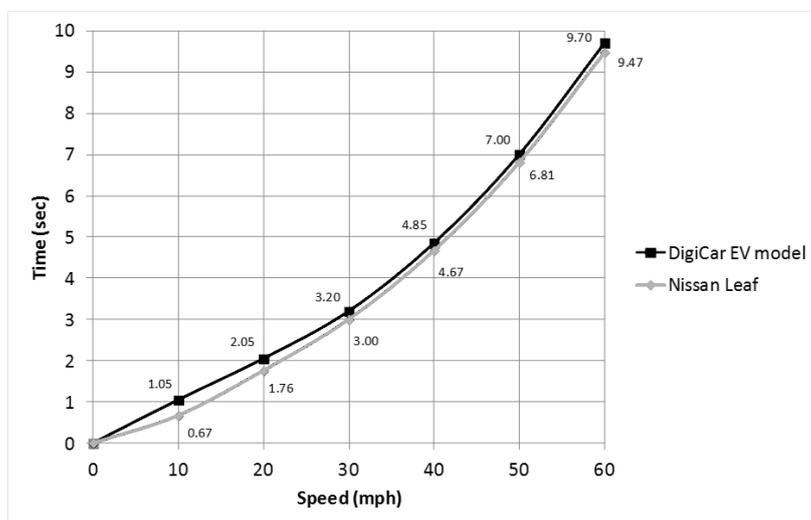
Figure 2: A comparison of the acceleration performance of the Nissan Leaf and the DigiCar EV model (acceleration times for the Nissan Leaf obtained from MyNissanLeaf.com)
