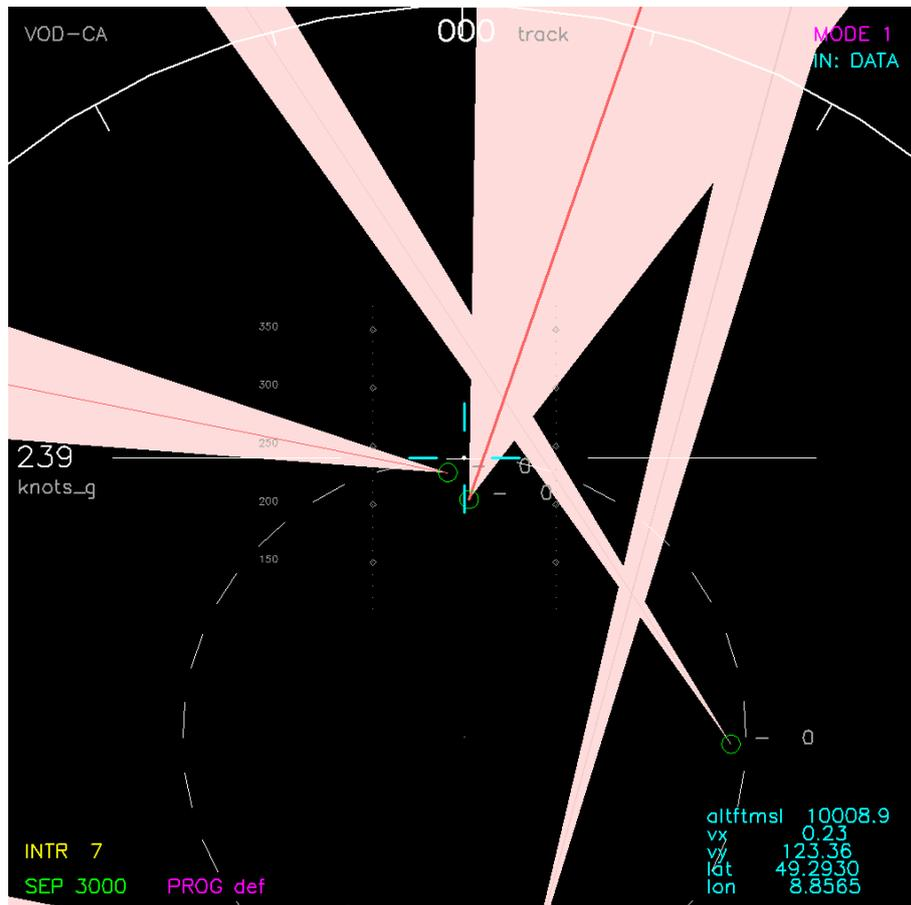
Figure 1. Velocity-Obstacle based Display for Collision Avoidance (VOD-CA)
