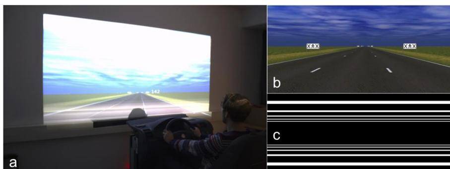
Figure 2: The experimental apparatus, a.) driving box at the Technische Universität Berlin, b.) driving scene from the Lane-Change-Task (Mattes, 2003), c.) overlay projection of moving transverse lines.
