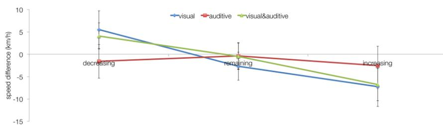
Figure 4: Mean speed differences between treatment and baseline drive as a function of the flow rate for each modality show that there was only an effect on the driving speed when the transverse lines were visually (included in multimodal) presented, an auditory presentation had no effect at all.
