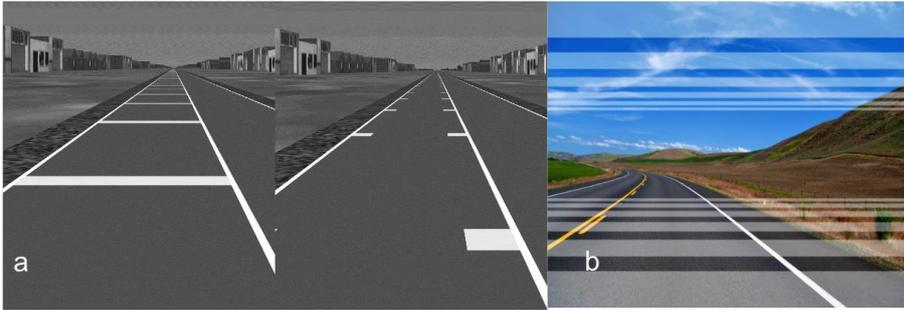
Figure 1: a.) Special road markings, from Godley et al. (1999), increase the optical flow rate in the peripheral view and consequently the perceived speed of the driver. b.) Moving transverse lines for the upper and lower peripheral area on the windshield as a possible information presentation for manipulating the perceived and consequently the driven speed.
