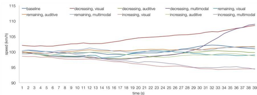
Figure 3: Mean trajectories of the treatment phase for each treatment, driving speed in-/decreased when moving transverse lines with a de-/increasing flow rate where whether visual or multimodal presented to the drivers.
