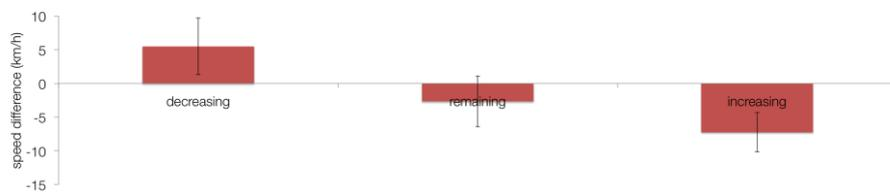
Figure 5: Mean speed differences between treatment and baseline drive caused by visually presented transverse lines show that a decreasing flow rate increases the speed about 5.5km/h (SEM=4.21), a remaining flow rate decreases the speed about 2.7km/h (SEM=3.76), and an increasing flow rate decreases the speed about 7.2km/h (SEM=2.94) on average.
