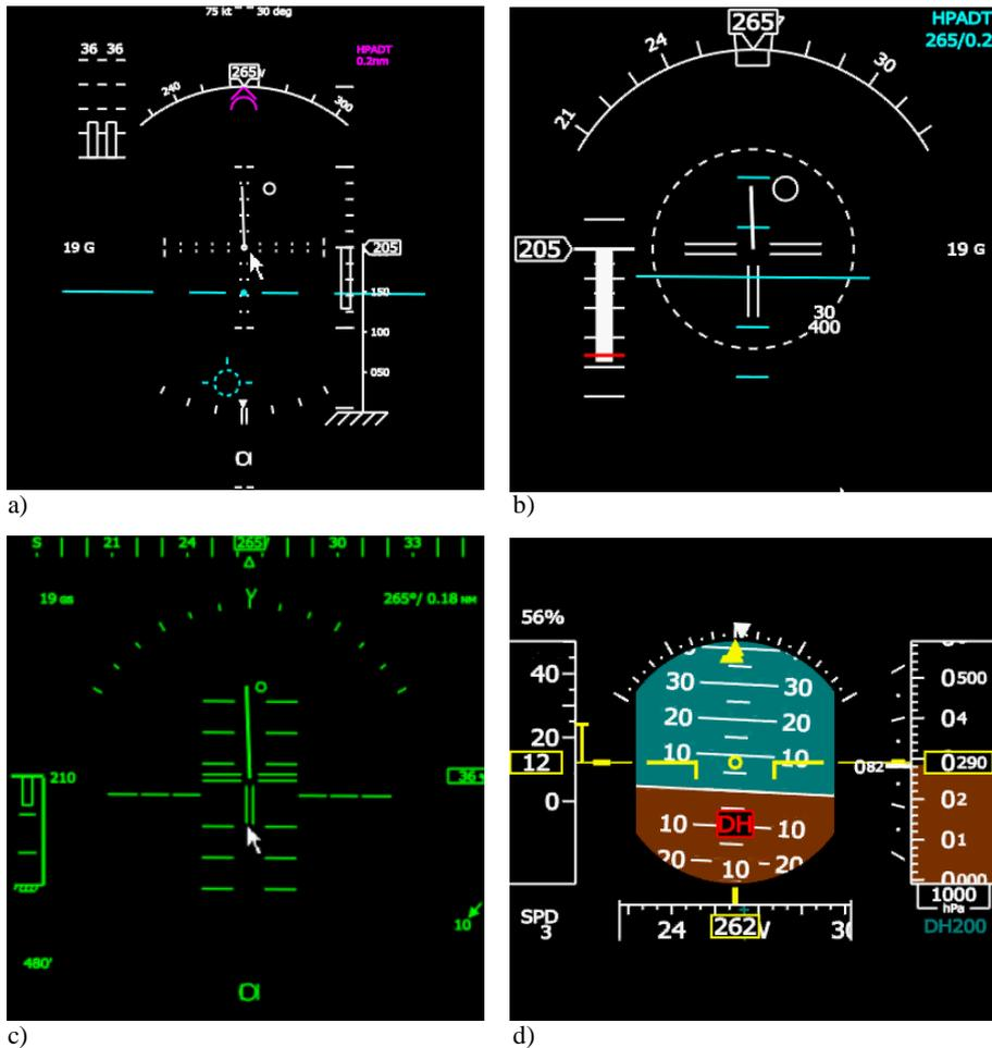
Figure 4. Symbology sets used in the experiment: a) BOSS, b) DEVILA, c) JEDEYE, d) PFD as control condition
