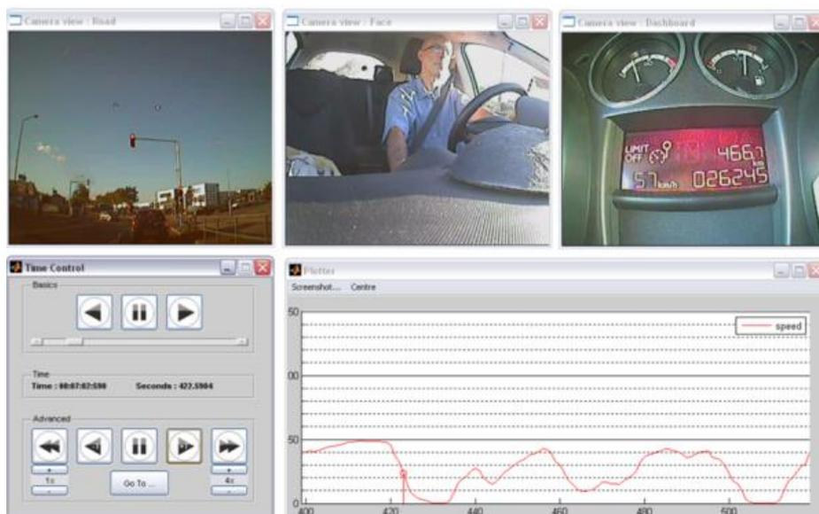
Figure 1: View of the three cameras and speed recording by the DAS
