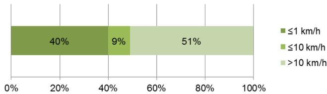
Figure 18: Overall distribution of handlings depending on car movement (mean speed during handling).
