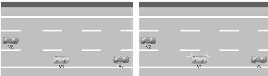
Figure 7: Operationalization of independent variable V2 lane change indication. Left = no indication; right = indication at TTC V2-V1  $\approx$  8.5 - 6.6 sec.
