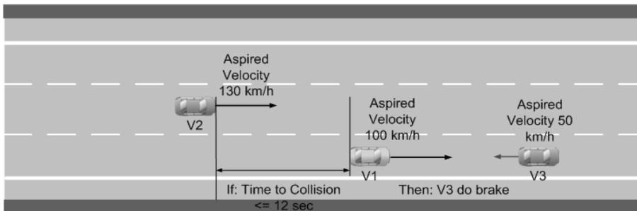
Figure 5: Triggering of a situation in which two agents can interfere
